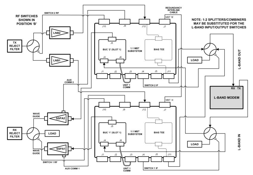
Figure C-1. Dual-Base Chain Redundant Operation
