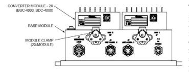
The Base Module for the MBT-4000 system – which provides the M&C, Power Supply, and Reference interfaces – may be located near or on the antenna. Guide pins and mechanical clamps keep the bandspecific BUC and BDC modules in place on top of the Base Module.
