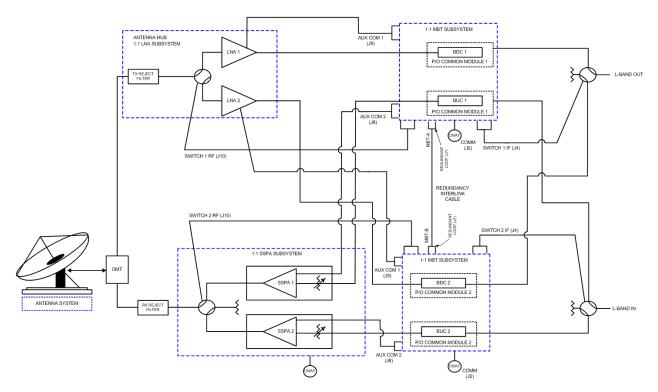
Figure 1-3. Operational Diagram for Dual-Base (Chain) Redundancy Option
